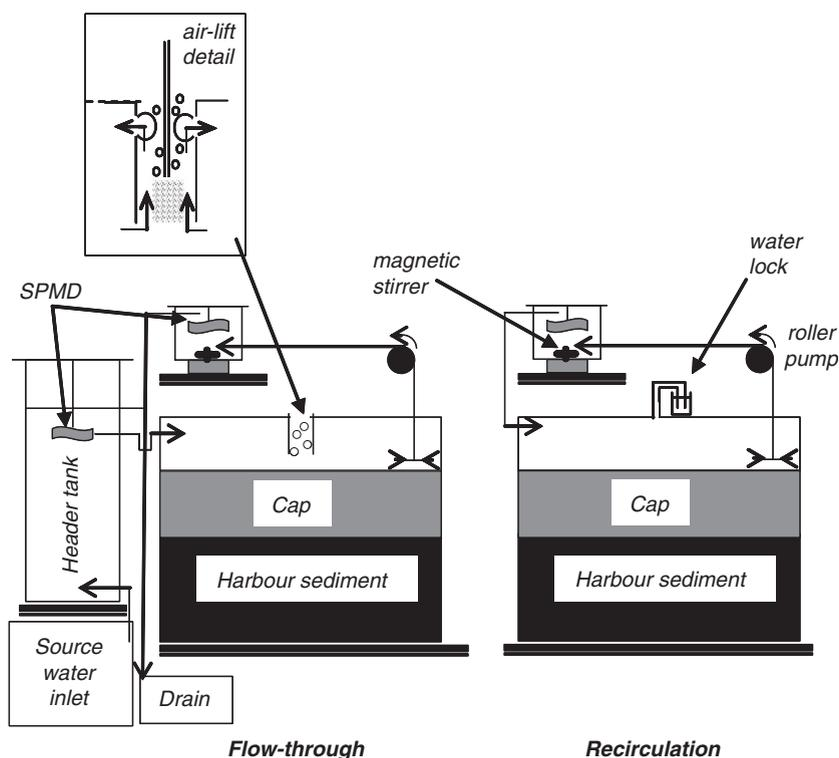
Fig. 1. Schematic drawing of the set-up during flow-through (left) and recirculation (right) measurements. Flags illustrate SPMDs in header tank and sampling cells.
